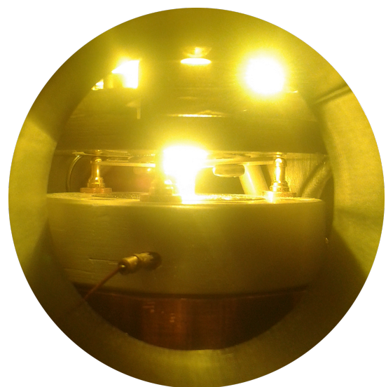
Black diamond high-temperature solar cell under characterization
